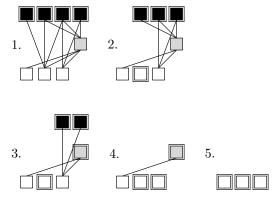
Fig. 2: Evolution of the decoding process of an example 3-block message. Squares with double-boundaries represent blocks that are known (recovered).
