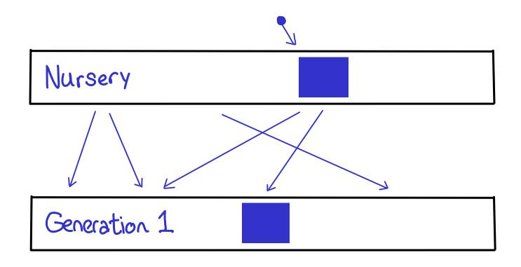
To talk about write barriers, we have to first go back to our picture of generations in the heap, and recall the invariant we imposed, which is that pointers are only allowed to flow from the nursery to the first generation, and not vice versa.
