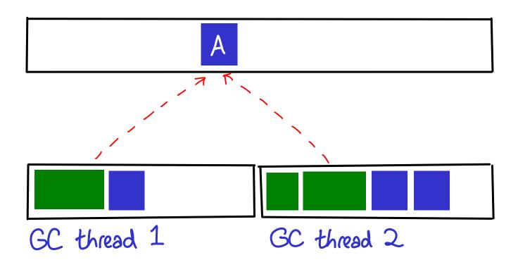
In an ideal world, only one of the threads would actually evacuate the object, and the other thread would update its pointer to point to its sole copy. Unfortunately, to do this, we'd have to add synchronization here. That's a BIG DEAL; most accesses to the heap here have no races and we really don't want to pay the cost of synchronization.
