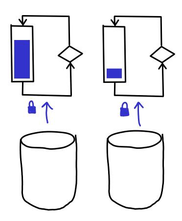
If a core runs out of work to do, it releases the HEC and goes to sleep.
