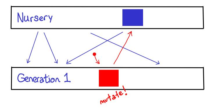
When mutation comes into the picture, there's a problem: we can mutate a pointer in an old generation to point to an object in the nursery.
