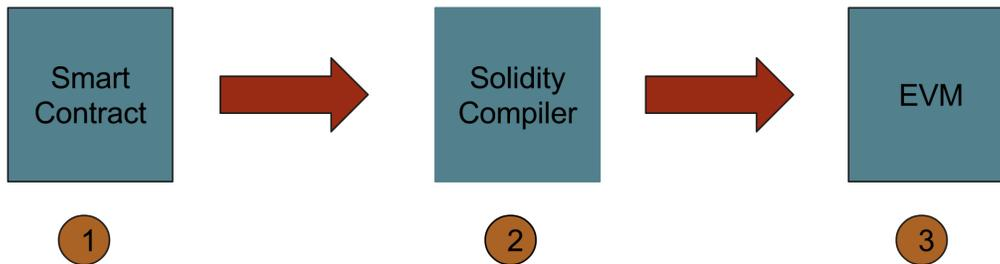
**Figure 4.** Steps to Deploy a smart contract on blockchain 1) create a smart contract in solidity, 2) compile and generate byte code and 3) deploy the contract on blockchain
