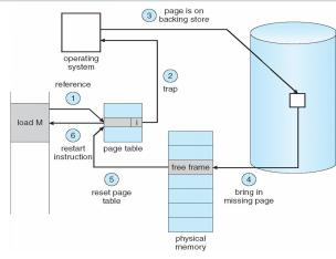
Use disk to simulate larger virtual than physical mem
