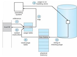
Use disk to simulate larger virtual than physical mem
