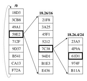
Figure 3-4: Peer selection on validated nodes. Shown is a lookup on key 541A, resulting in the node tuple with hash value 61D1, which belongs to the domain 18.26.4/24.
