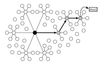
Figure 3-5: Mimic topology and traffic flows for k=3: each node has  $\kappa\approx 6$  mimics (shown connected by solid lines); a node establishes its tunnel over mimic links (arrows in bold) and completes it with a random PNAT (dotted line). Nodes inject cover traffic with data traffic to yield a uniform total traffic  $\mathcal T$  that flows bidirectionally over the solid lines. All packets on these links are pair-wise encrypted and padded to the same size.
