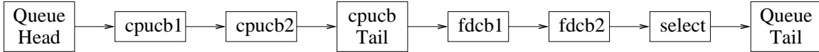
Figure 3-3: The callback queue structure in libasync-mp . cpucb() adds new callbacks to the left of the dummy element marked “cpucb Tail.” New I/O callbacks are added at “Queue Tail.” The scheduler looks for work starting at “Queue Head.”
