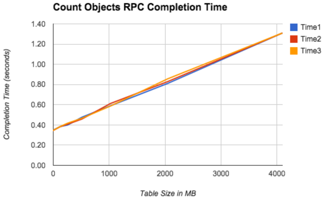
Figure 3. Count RPC completion time on a single server, varying the amount of data in the hash table. Even with 1 object in the hash table there is a fixed cost of searching every hash table bucket.
