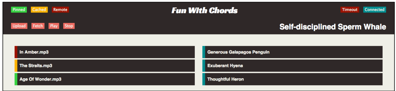
Figure 1: The FWC client. The local file index consists of one remote file record, one cached file record, and one pinned file record (left). There are three other nodes in the group (right).
