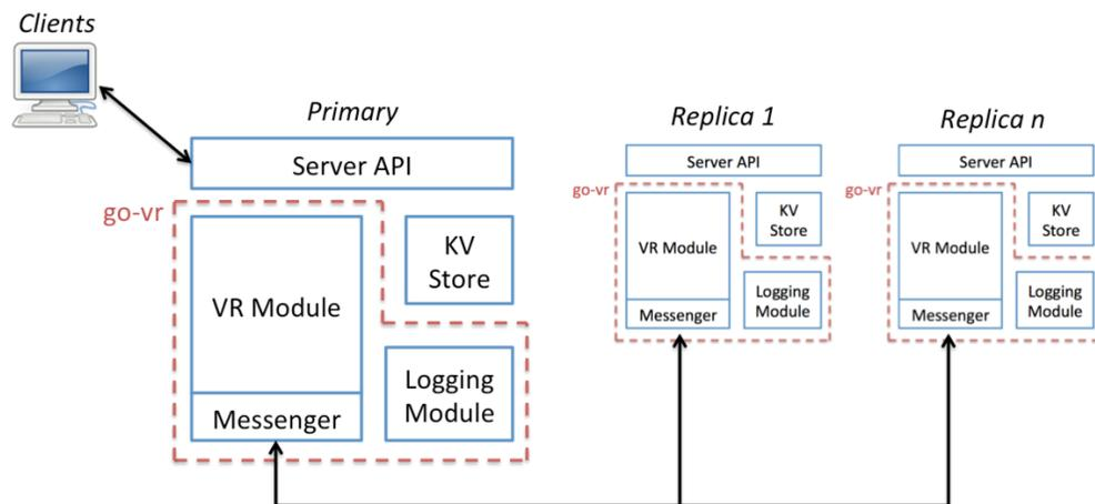
Go-VR was designed to be easily integrated with other distributed system and it mainly comprises of a VR module, an inter-node messaging module and a logging module, as shown in figure 1. Through a set of provided APIs, services that need replicated operations communicate with Go-VR by registering a callback function and passing in serialized messages for replication.
