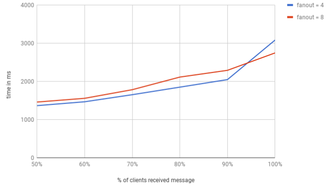
Fig. 5. Testing message propagation latency for different fanout values with no faulty nodes.
