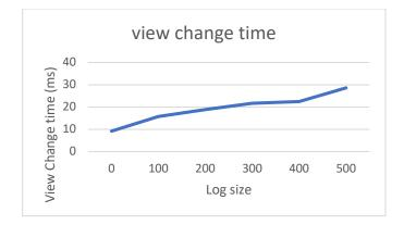
To answer question 3, I ran a client to periodically send requests to a 5-node cluster and at various points of time, triggered a view change by bringing down the primary. The time taken to complete a view change increased linearly as the size of the logs increased. This is attributed to the size of the messages being transmitted during a view change and only goes to show that it is crucial to limit the size of the messages for VR to remain performant over time.
