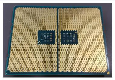
4094 pins: both memory controller and 128 lanes PCIe directly on chip!
