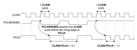
Figure 2-2 PCLKENDBG with CLKIN:PCLK ratio changing from 3:1 to 1:1
