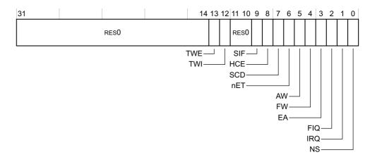
Figure 4-101 SCR bit assignments
