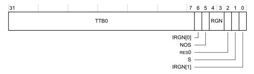
Figure 4-111 TTBR0 bit assignments, TTBCR.EAE is 0
