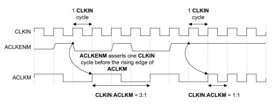
Figure 2-3 ACLKENM with CLKIN:ACLKM ratio changing from 3:1 to 1:1
