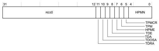
Figure 4-34 MDCR\_EL2 bit assignments
