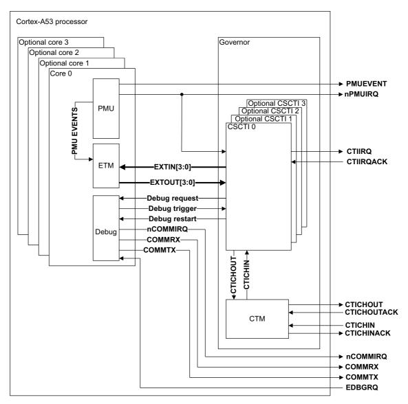
Figure 14-1 Debug system components
