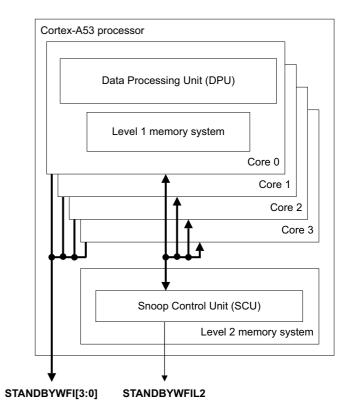
Figure 2-12 STANDBYWFI[3:0] and STANDBYWFIL2 signals
