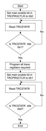
Figure 13-2 Programming ETM trace unit registers
