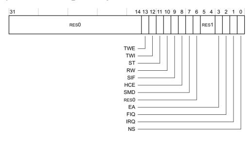
Figure 4-38 SCR\_EL3 bit assignments
