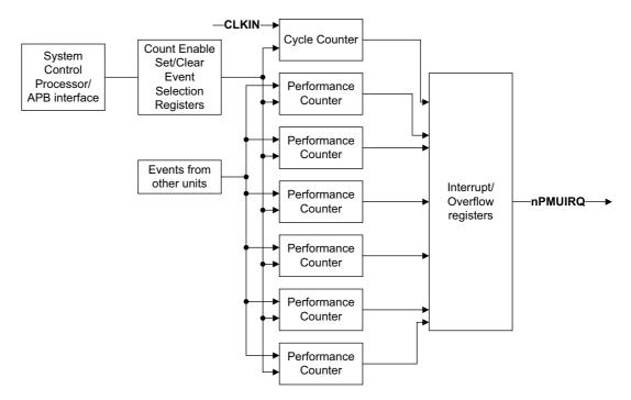
Figure 12-1 PMU block diagram
