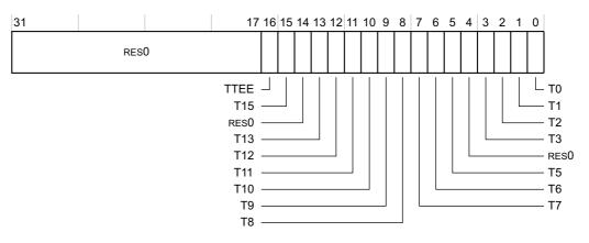
Figure 4-120 HSTR bit assignments
