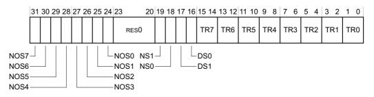
Figure 4-133 PRRR bit assignments
