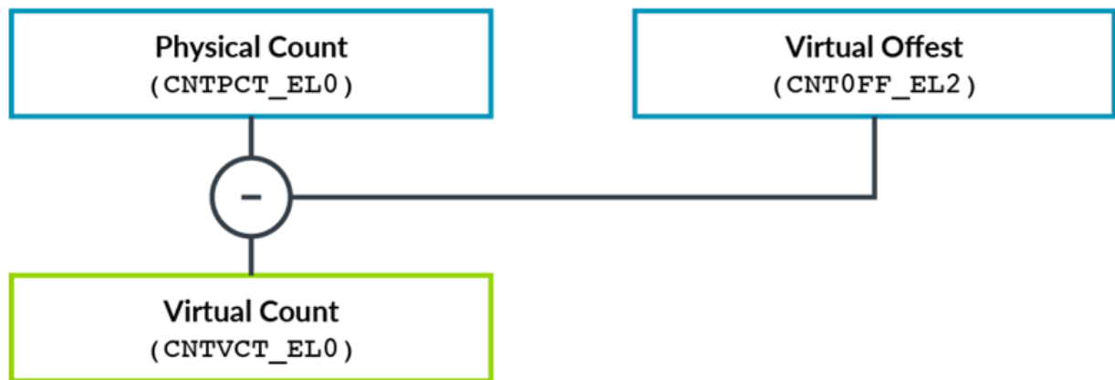
Figure 7-3: How the virtual counter is generated
