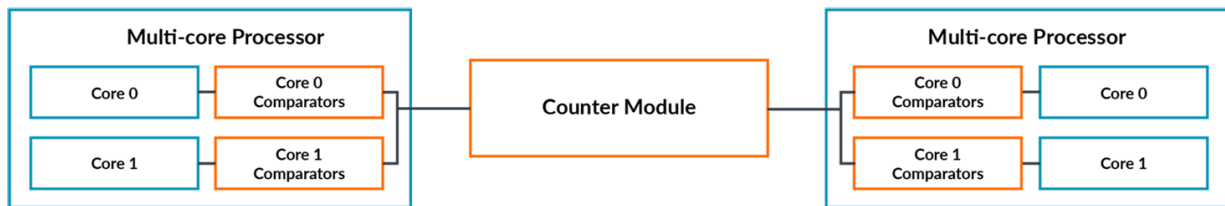
Figure 7-1: System counter module and per core comparators
